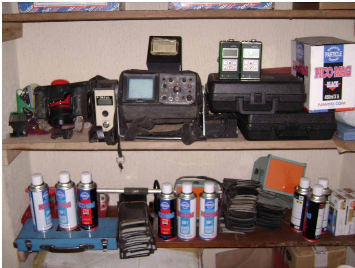
Ultrasonic Set, Ultrasonic Gauges, Magnetic Particles Inspection and Dye Penetrant Inspection Kits
