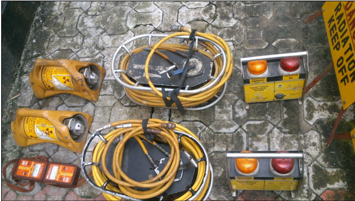
Isotope Container Delta 880, Control Unit, Radiation Revolving Alarm and Survey Meter.
